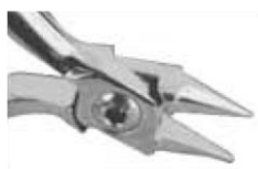
A-DTL-3157 Wire bending and loop forming pliers Angled (Bird beak) ● 0.30 mm to 0.50 mm (.012" to .020") ■ Max 0.56 mm x 0.71 mm (.022" x .028")
