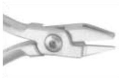
A-DTL-3169 Aderer Clamp three jaw Wire bending plier for contouring and Bending wire up to .30"/.76 mm
